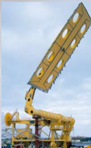
Special cylinders in hydraulically manoevrable cover equipment.
