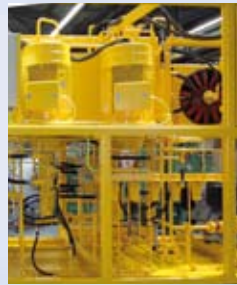
Power unit for undercarriage operation
