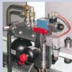
Diaphragm accumulator for damping in the lubrication system.
