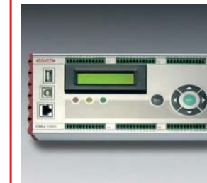
ConditionMonitoring Unit CMU 1000 for recording, manipulating and evaluating measured data.
