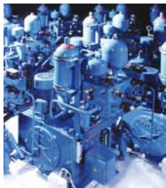
Wind turbine: Hydraulic power unit for braking function and yaw adjustment
