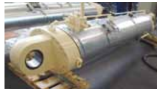
Bucket wheel excavator: Hydraulic cylinder
