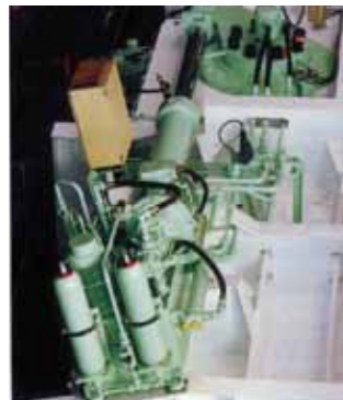
Hydraulics for ship stabilisers
