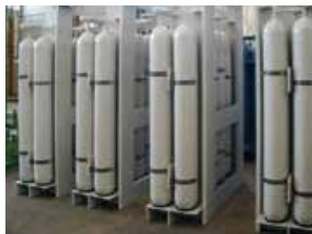
Accumulator station for press line
