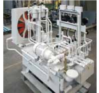
Cement mill: Lubrication system
