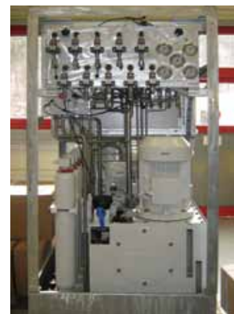
Wind turbine: Hydraulic power unit for braking function and yaw adjustment
